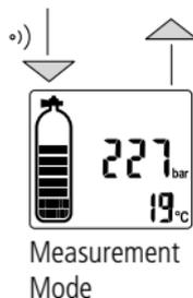
🔍 The number of bars shown in the tank symbol correlates to the relation between the actual pressure and 200 respectively 300 bar, depending on the measured maximum pressure. If the maximum pressure exceeds 250 bar (3600 psi) the number of bars is displayed as a proportion of 300 bar (4500 psi). With a maximum pressure of less than 250 bar (3600 psi) the number of bars is proportional to 200 bar (3000 psi).
