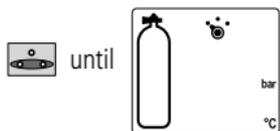
→ The Digital Pressure Gauge has to be in the User Mode (see page 10). Bridge the contacts B and S until the symbol for the Set Up Mode
