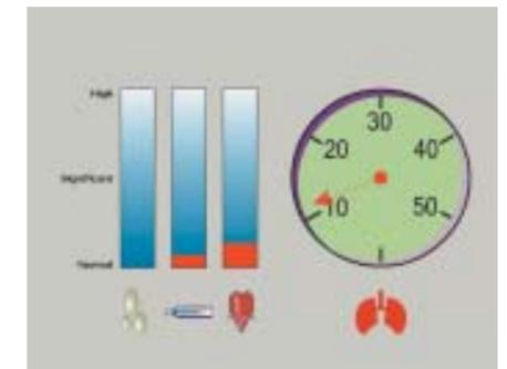
After a dive, the data from the Smart COM can be downloaded to Personal Computer with the Smart TRAK software that is included with the Smart COM. The actual rate of breathing is displayed in l/min, as is the workload level. Also displayed is microbubble buildup and temperature.
