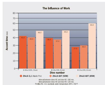
Earlier mathematical models assumed a mean workload output of 50W. With the ZH-L8 ADT MB model, even at level 0, if workload is increased to 85W then on a (15m) 50ft dive the ascent time is increased from 30 to 60 mins.
