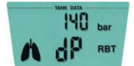
At the conclusion of a dive the Smart COM displays the "differential pressure". This value represents the gas that is consumed during the dive. Also displayed are any warnings that may have occurred throughout the dive, in this example both RBT and Workload warnings are displayed.
