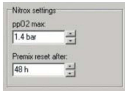
With Smart TRAK software the Nitrox diver can change the maximum partial pressure of oxygen on both the Smart COM and the Smart PRO. For a diver who anticipates diving on the same nitrox mixture for a number of dives, with Smart TRAK it is possible to set the mixture reset to the default air (21% O<sub>2</sub>) for an interval of up to 48 hours after a dive.
