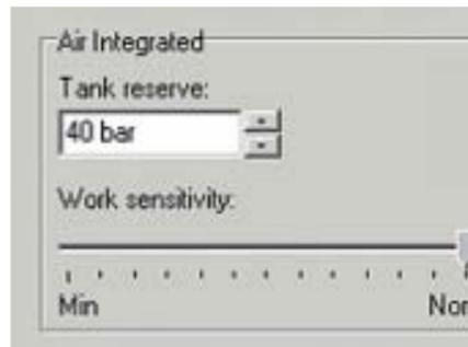
With the Smart TRAK software that is supplied with the Smart COM, the sensitivity of the workload setting can be set by the diver according to their own level of fitness.
