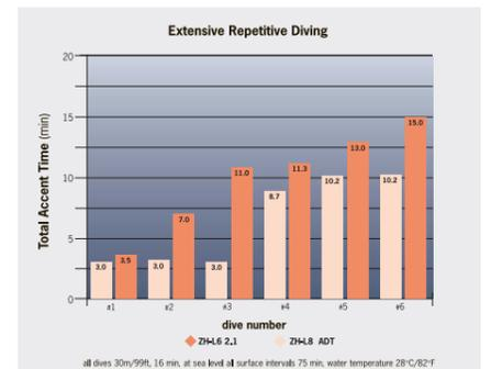
In comparing earlier fixed models with the ZH-L8 ADT MB model, even at level 0 the no decompression times for the first ascent are nearly identical, whereas for the following dives the total ascent times are greater by up to a factor of four.
