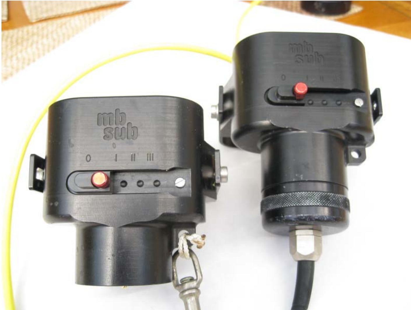
Position 1: Half power single bulb. Position 2: Full power single bulb and Position 3: Full power dual bulb. As before the head is attached via a double Oring sealed connector and power is transferred through a gold plated coax type plug.
